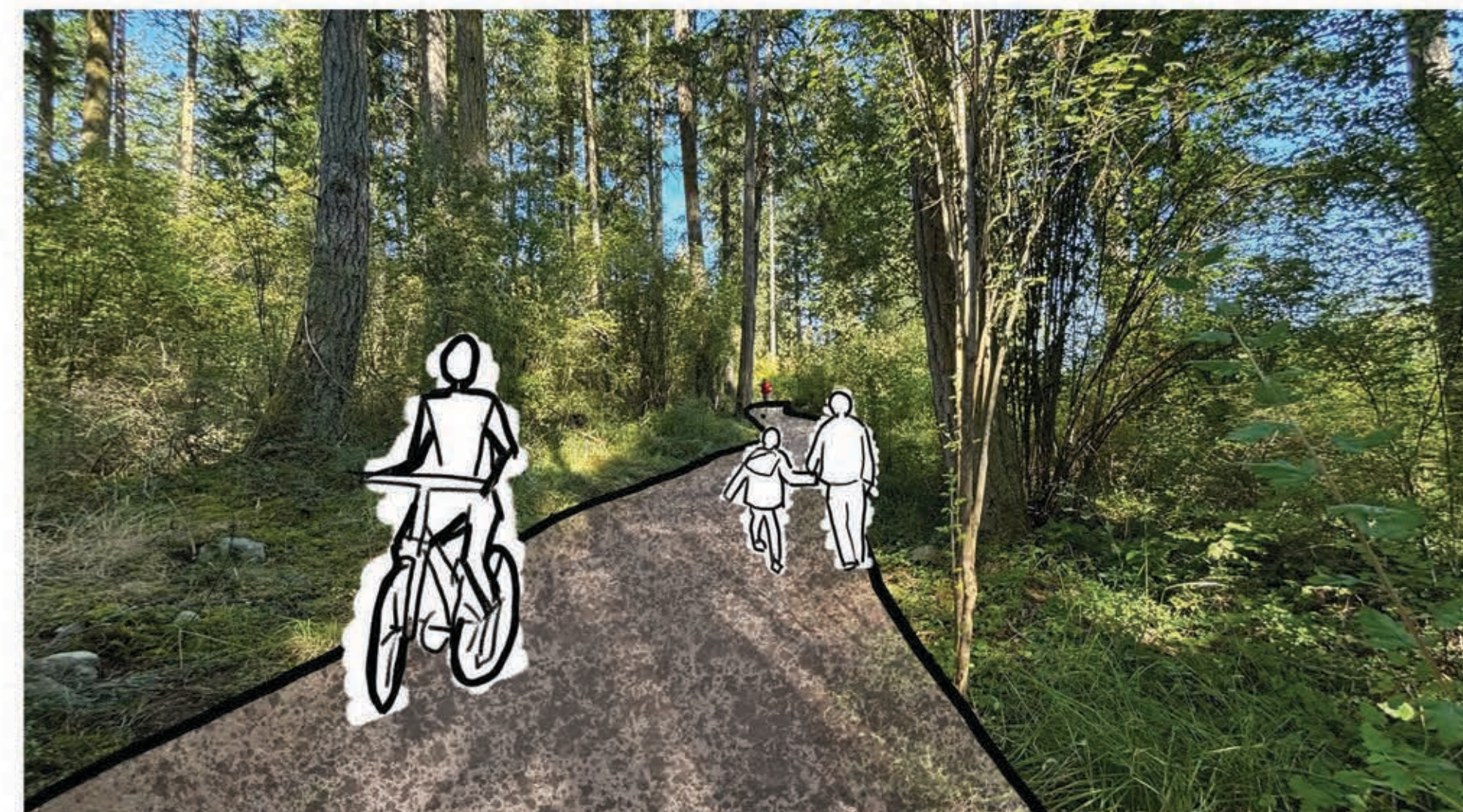
PROPOSED EAST TRAIL - CRUSHED ROCK TRAIL 8' WIDE WITH 1' SHOULDER EACH SIDE
